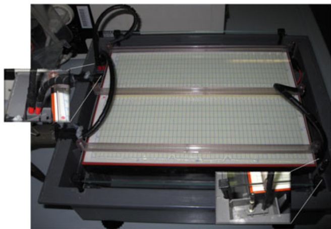
Figure 3. Electrophoretic chamber (Multiphor II) with the three electrodes correctly plugged in. Note the connection of the two anodes to the socket.
